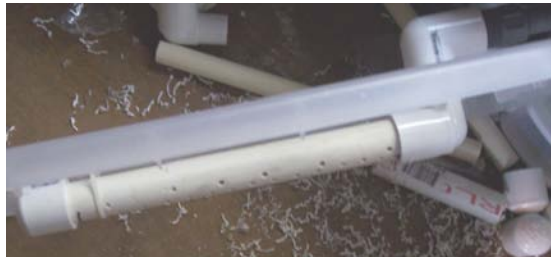
Figure 5 Spray bar mounted on lid
