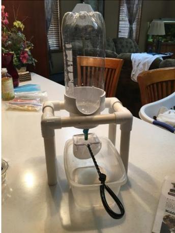
Lengths of 3/4" PVC pipe for Double Aquarium Brine Shrimp Hatcher – (2) 3" for sides, (2) 7.5" for front and back, (4) 3" for legs.
